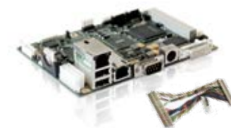
JRExplus-DC with memory (if needed flat panel cables)
