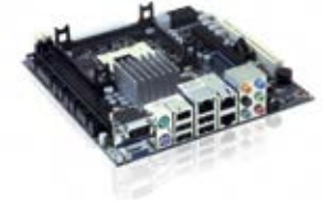
KTGM45/mITX with heatsink and socketed CPU
