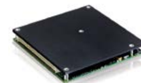
COM Express® compact with memory and heatspreader
