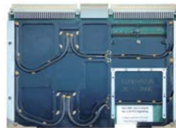
PowerNode5 with heat pipe
